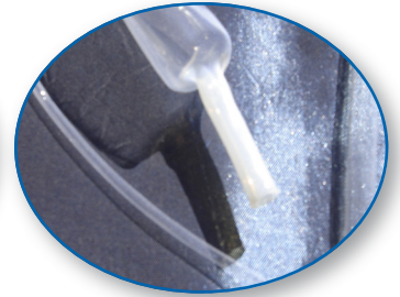
TRPTFE4X PTFE heat shrink tubing 4:1 Contraction Working temperature -70° C to 260° C
