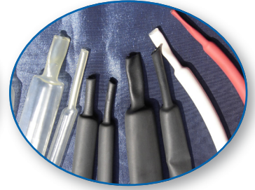
TRPFAH Polyolefin heat shrink tubing Thin wall / With adhesive 3:1 Contraction Working temperature -45° C to 125° C
