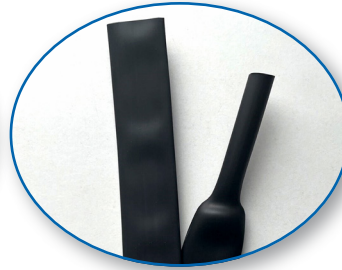
TRPF200°C Polyolefin heat shrink tubing Thin wall / Without adhesive 2:1 Contraction Working temperature -55° C to 200° C
