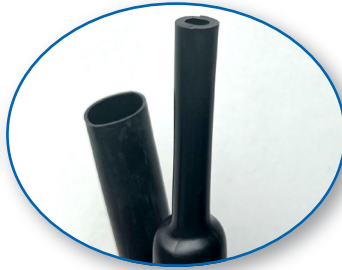
TRPM-S/A Polyolefin heat shrink tubing Medium wall / Without adhesive 3:1 Contraction Working temperature -45° C to 110° C
